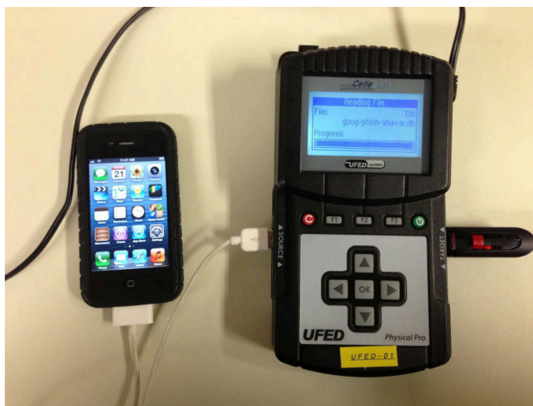
A Cellebrite Universal Forensics Extraction Device (UFED) extracting data from an iPhone 4S, 2013.
