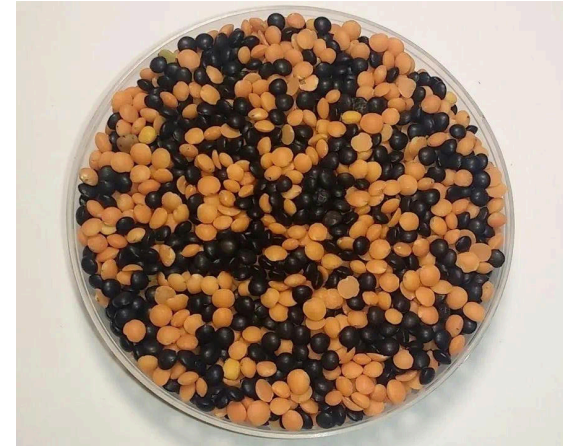
A mixture of red and black lentils with a complex pattern. Electronic devices can be immersed in the mixture so that when they are accessed, the pattern changes.
