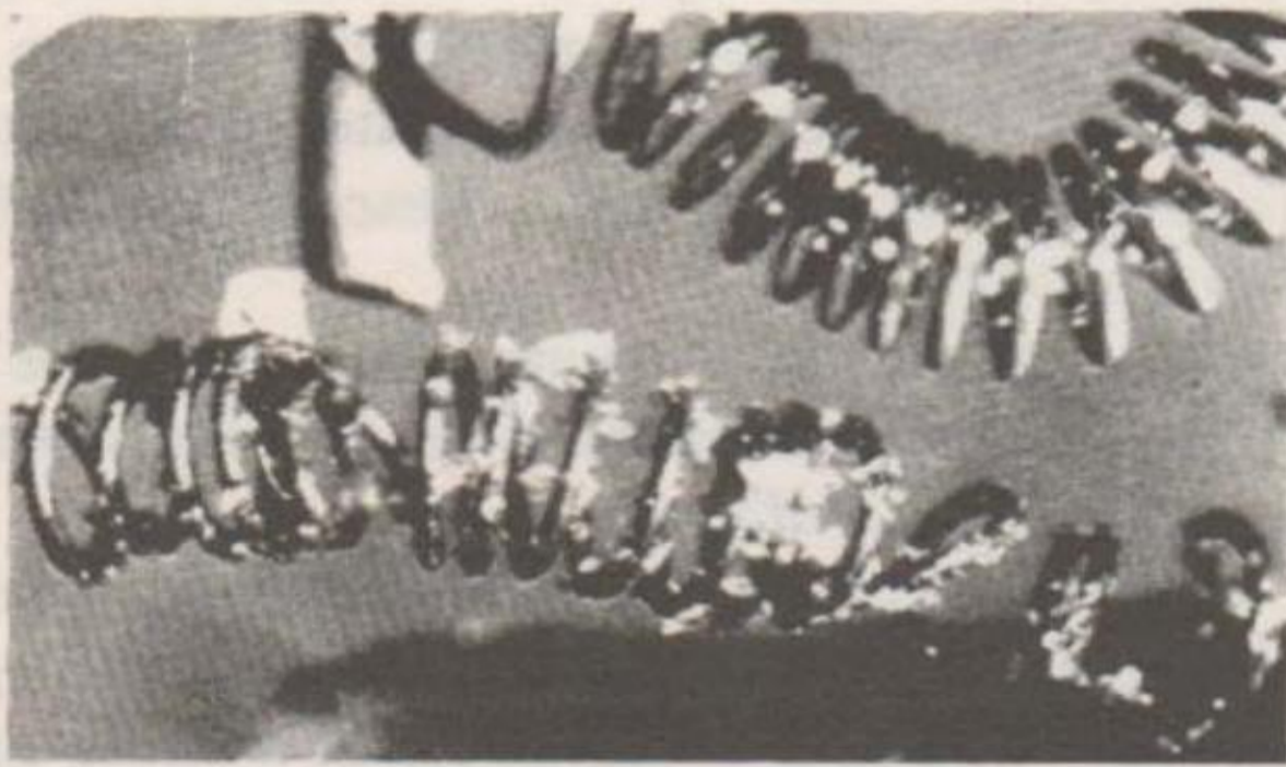
Filament of a car headlight. The bulb was broken in an accident. The adhering glass shows that the filament was hot, i.e. that the lamp was alight.
