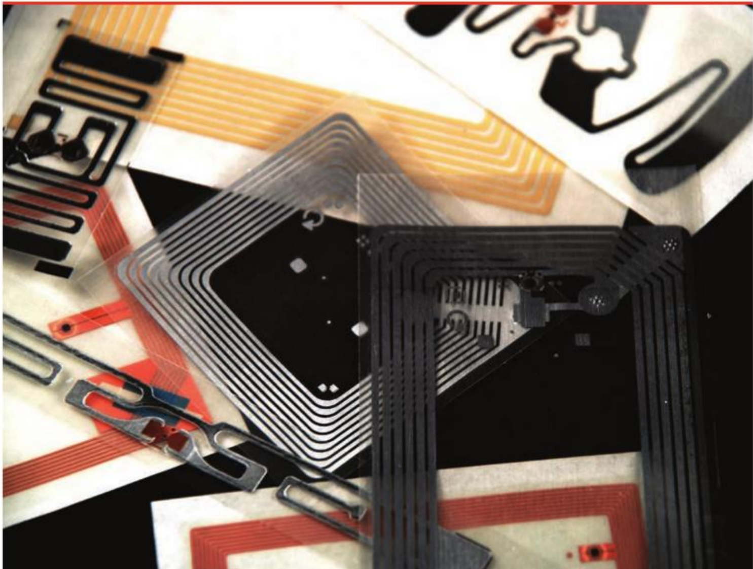
RFID tags, which come in many shapes and sizes (Source: © iStockphoto.com/albln)
