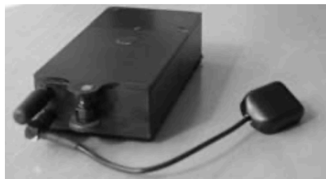
Right: GPS transmitter from the BKA (2007), GPS antenna separately.
