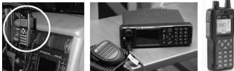
TETRA devices currently in use: hand-held device permanently installed in the car; MRI (base unit) from Motorola; HRT (hand-held) from Sepura.
