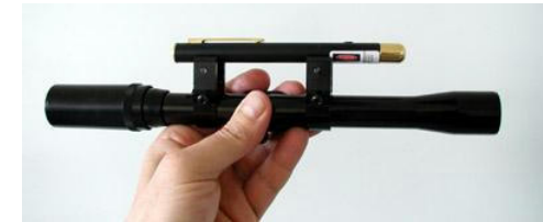
Simple laser / rifle scope system.
