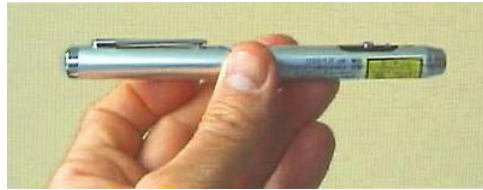
Inexpensive laser pointer (1 mW, 650 nm red).
