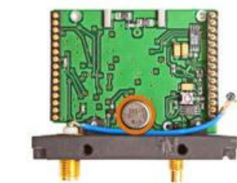
Module providing RF transmission capabilities (other side)
