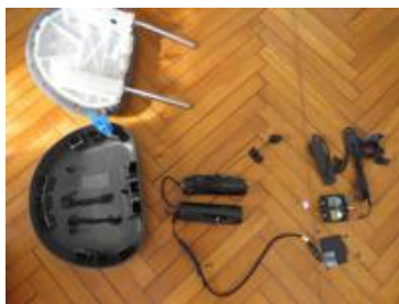
1: control unit; 2: batteries; 3: GPS antenna; 4: microphone; 5: SIM card
