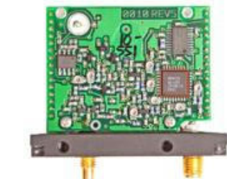
Module providing RF transmission capabilities
