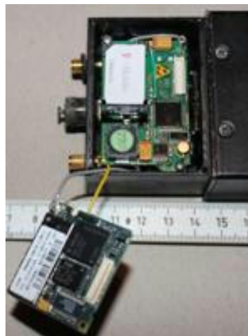
GPS tracker open with SIM card
