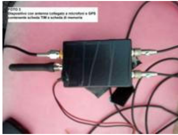
The device with an antenna connected to the microphones and GPS. It also included a SIM and memory card.
