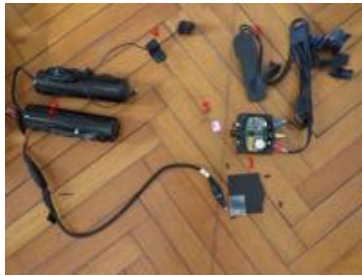
1: control unit; 2: batteries; 3: GPS antenna; 4: microphone; 5: SIM card
