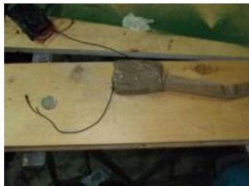
The device was like that when it was found. The microphone is next to the two euros coin and the antenna is at the other end.
