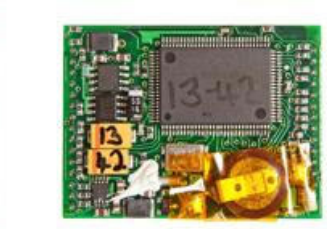
Module providing the GPS signal (other side)
