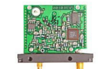
Module providing RF transmission capabilities
