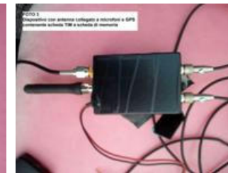
The device with an antenna connected to the microphones and GPS. It also included a SIM and memory card.
