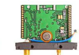
Module providing RF transmission capabilities (other side)
