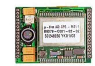
Module providing the GPS signal
