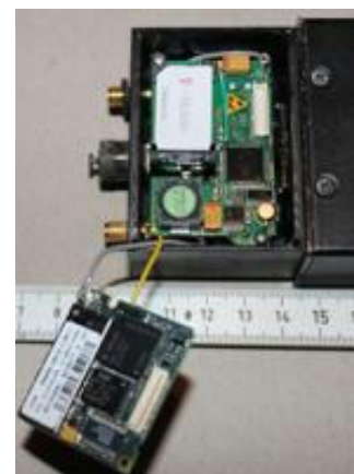
GPS tracker open with SIM card
