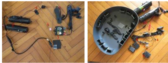
1: control unit; 2: batteries; 3: GPS antenna; 4: microphone; 5: SIM card 2: two batteries of the listening device; 4: microphones connected to the listening device; 6: dismantled listening device; 7: SD card
