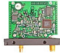
Module providing RF transmission capabilities
