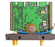
Module providing RF transmission capabilities (other side)
