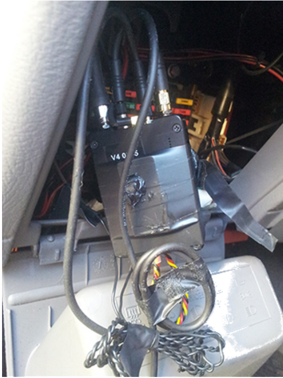
Microphones and a GPS tracker found in the fuse box of a car in Lecce, Italy, in December 2017 2 .
