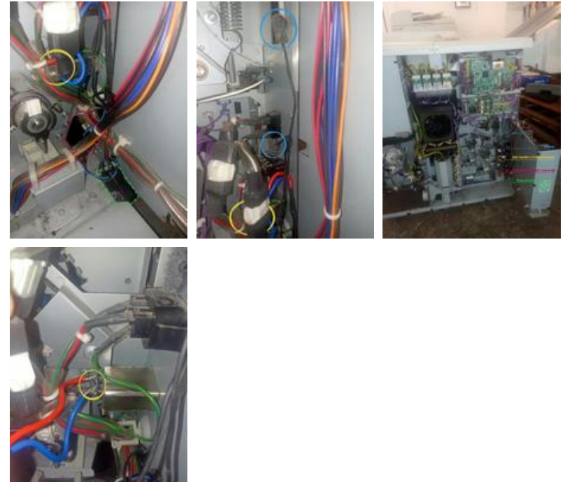
Blue: microphones; Yellow: wires soldered to the power supply; Pink: small box with SIM card + SD card; Green: transformer
