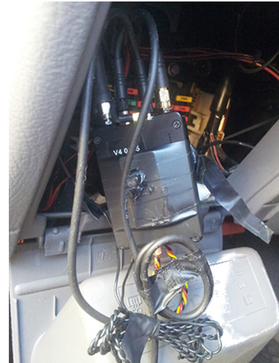
Microphones and a GPS tracker found in the fuse box of a car in Lecce, Italy, in December 2017 2 .
