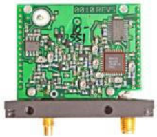
Module providing RF transmission capabilities
