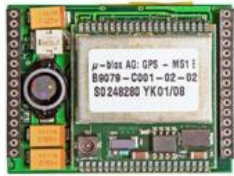
Module providing the GPS signal
