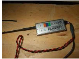
Detail of the emitting antenna with its cover
