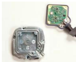
GPS antenna board
