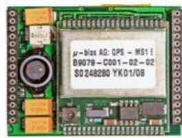
Module providing the GPS signal
