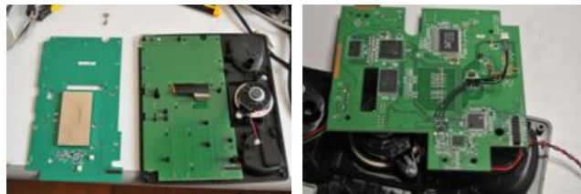
On the left: modified version of the phone largest circuit board (with surveillance device) without the battery pack. On the right: unmodified version.
