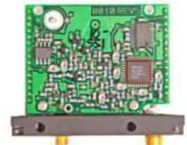
Module providing RF transmission capabilities
