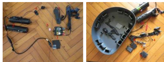
1: control unit; 2: batteries; 3: GPS antenna; 4: microphone; 5: SIM card 2: two batteries of the listening device; 4: microphones connected to the listening device; 6: dismantled listening device; 7: SD card
